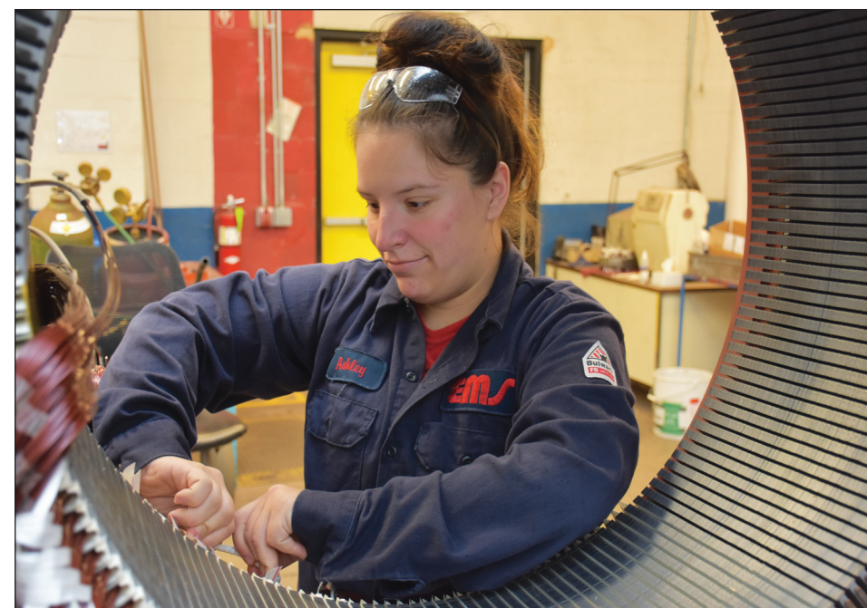
Ashley Rogal, Chief Rewinder at EMS rewinds a motor stator. The rewinding process takes more than three days.
